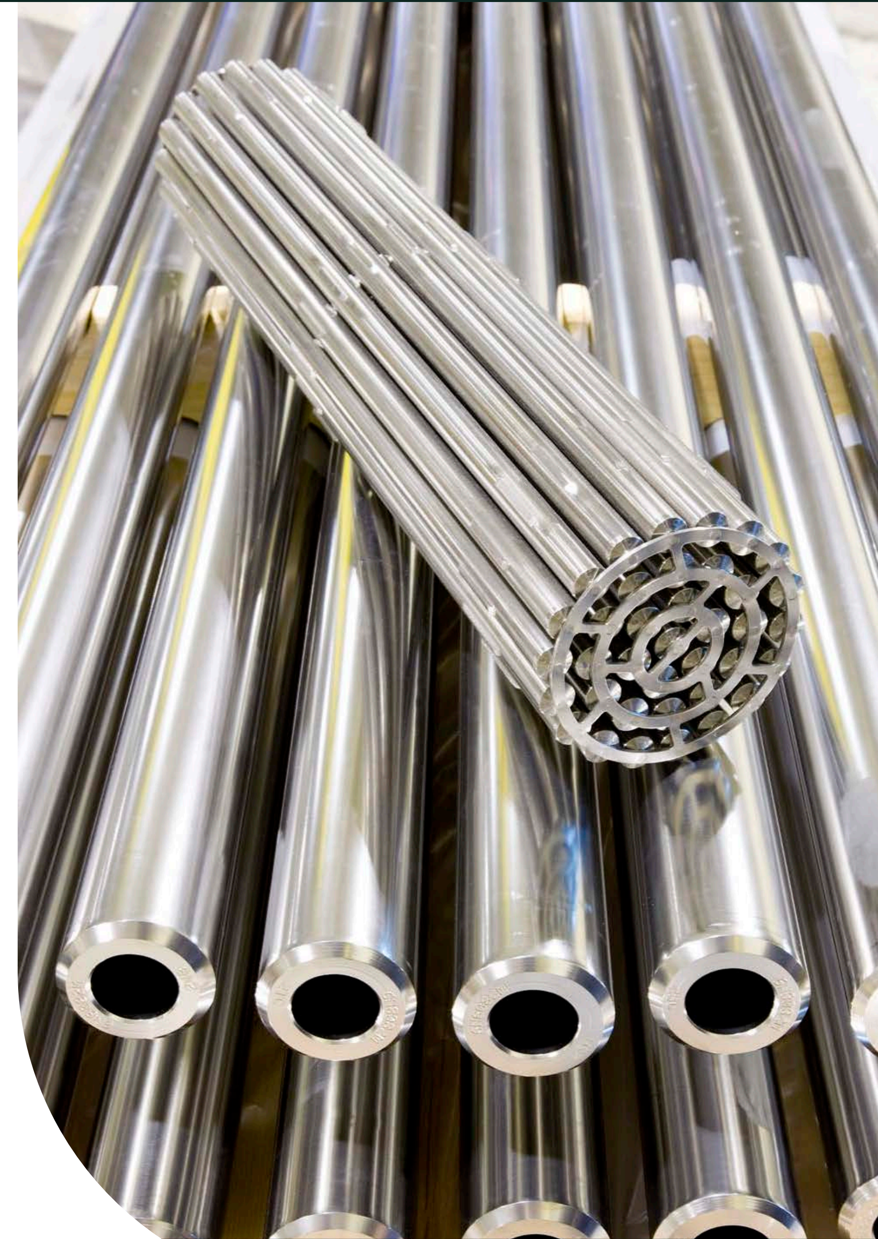
A uranium fuel rod for use in a CANDU reactor.
