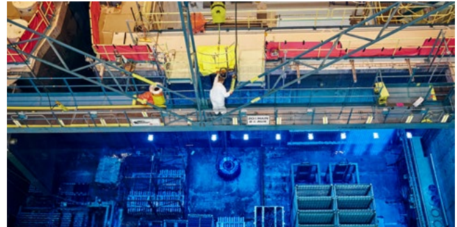
Once Co-60 rods are harvested from a reactor at Bruce B, they are separated into individual bundles underwater and loaded into specialized shipping containers for transport to Nordion for further processing before heading to an international market.
