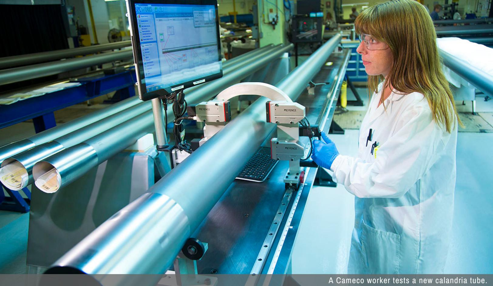
A Cameco worker tests a new calandria tube.
