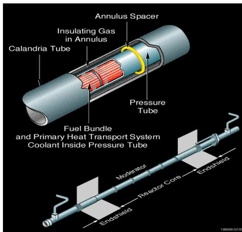
*Figure 3 - Section View of Fuel Channel Assembly*
