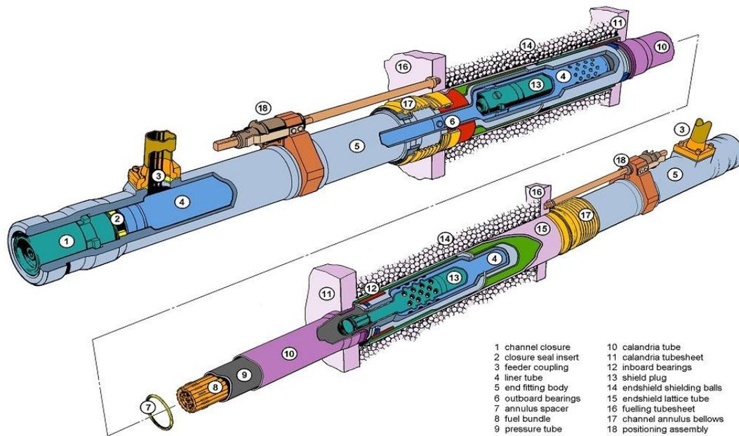
*Figure 4 - Detailed view of Pickering 5-8 Fuel Channel*
