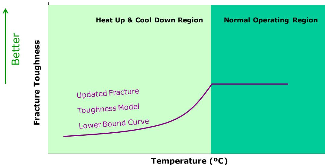
*Figure 8 - Updated Lower Bound Fracture Toughness Curve accounting for high Hydrogen Content*
