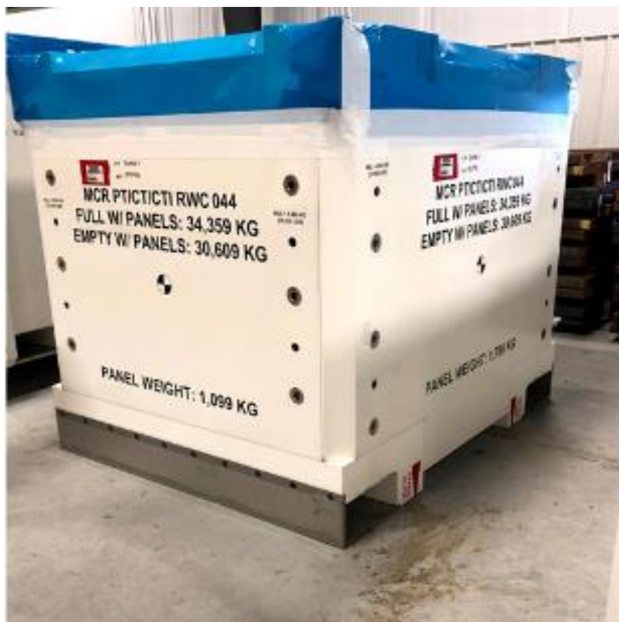
Figure 2-19: Photograph of a Major Component Replacement Retube Waste Container
