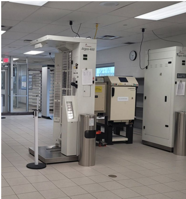
Figure 17: NSS-D Personnel Contamination Monitoring equipment
