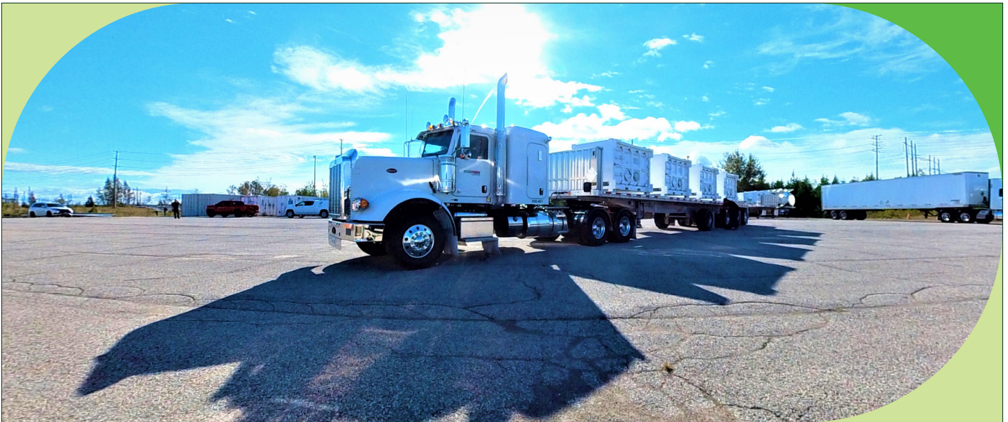
OPG's RMT transport truck and trailer loaded with low-level waste transportation containers
