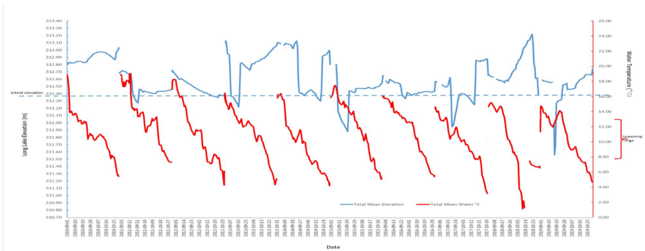
Figure 1 Water elevation (blue) and temperatures (red) for Long Lake for September through October (2010 to 2019). Dashed blue line represents the autumn drawdown intent (312.40m) identified in the WMP.
