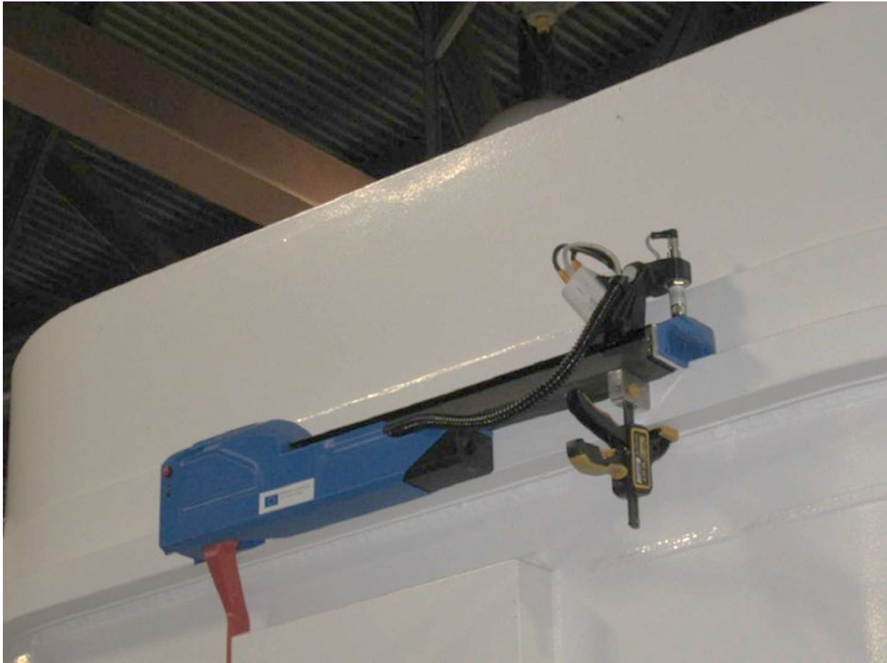
Figure 35: Laser Mapping Container Verification (LMCV)
