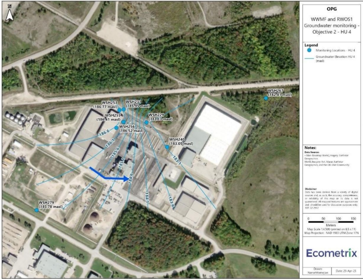
Figure 31: 2024 WWMF Middle Sand Aquifer Groundwater Contour Map
