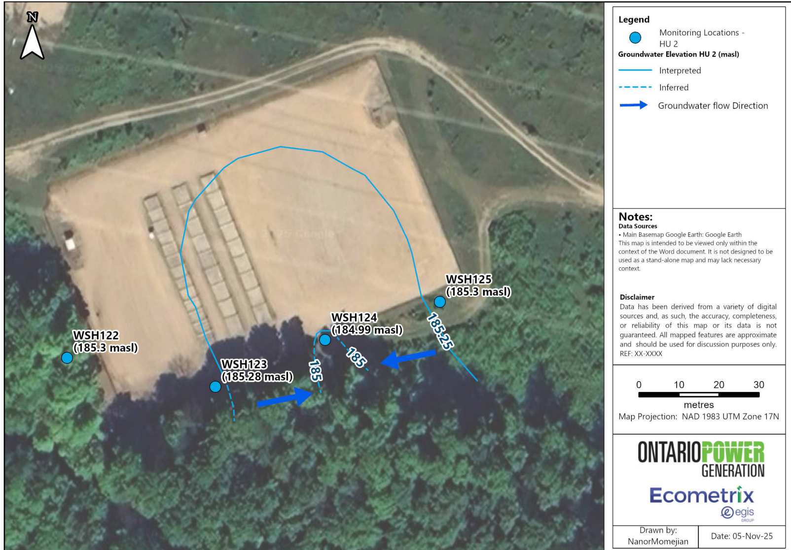
Figure 15: 2024 Native Sand (HU2) Groundwater Contours at RWOS1 based on April 17, 2024, measurements
