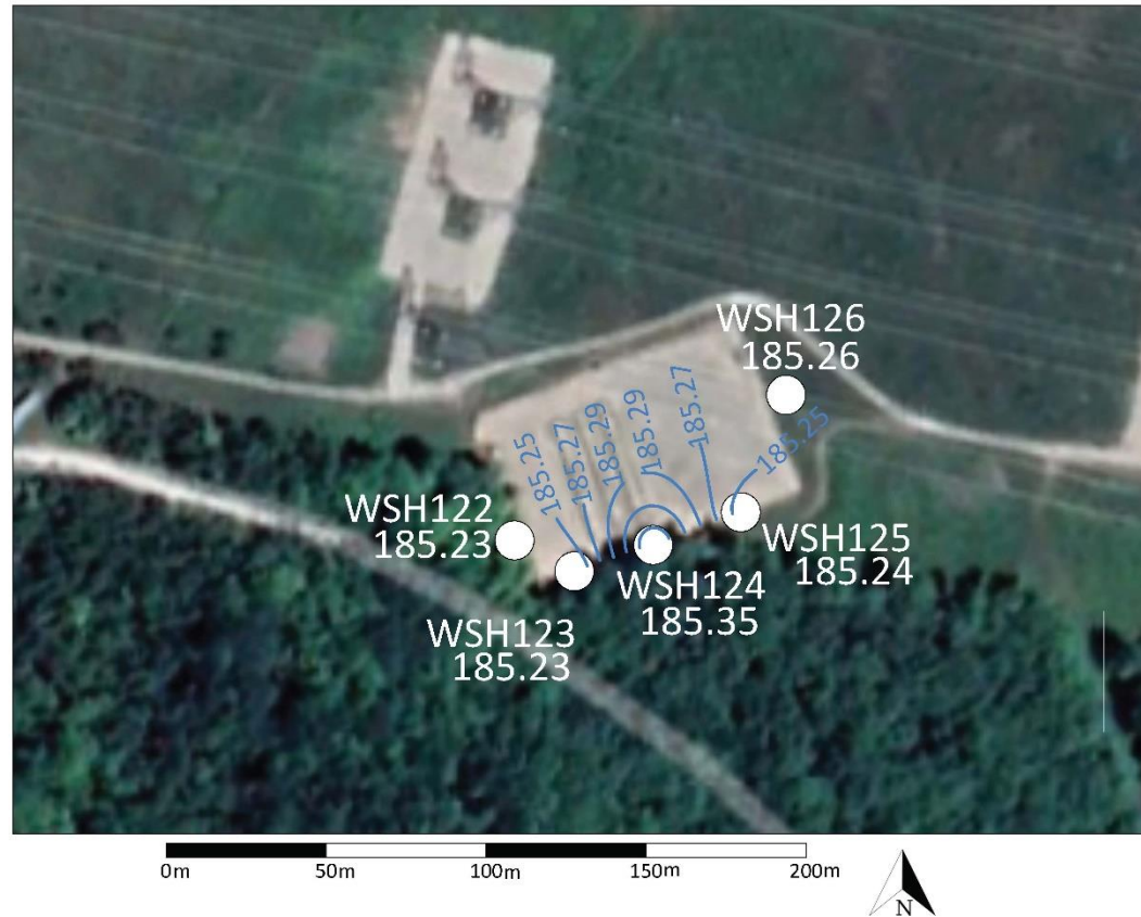
Note: Elevations and contours are reported in masl. Figure 15: 2023 Native Sand (HU 2) Groundwater Contours at RWOS1 based on May 15 th , 2023 measurements
