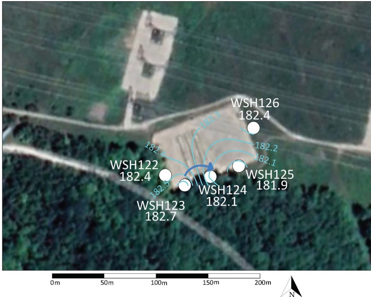
Figure 16: 2022 Q4 (HU 2) Groundwater Contours at RWOS1 (December 12, 2022). Note: Elevations and contours are reported in masl.
