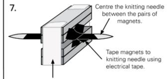
Tape magnets together using masking tape.
