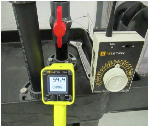
Simulated gamma meter and radiofrequency remote control
