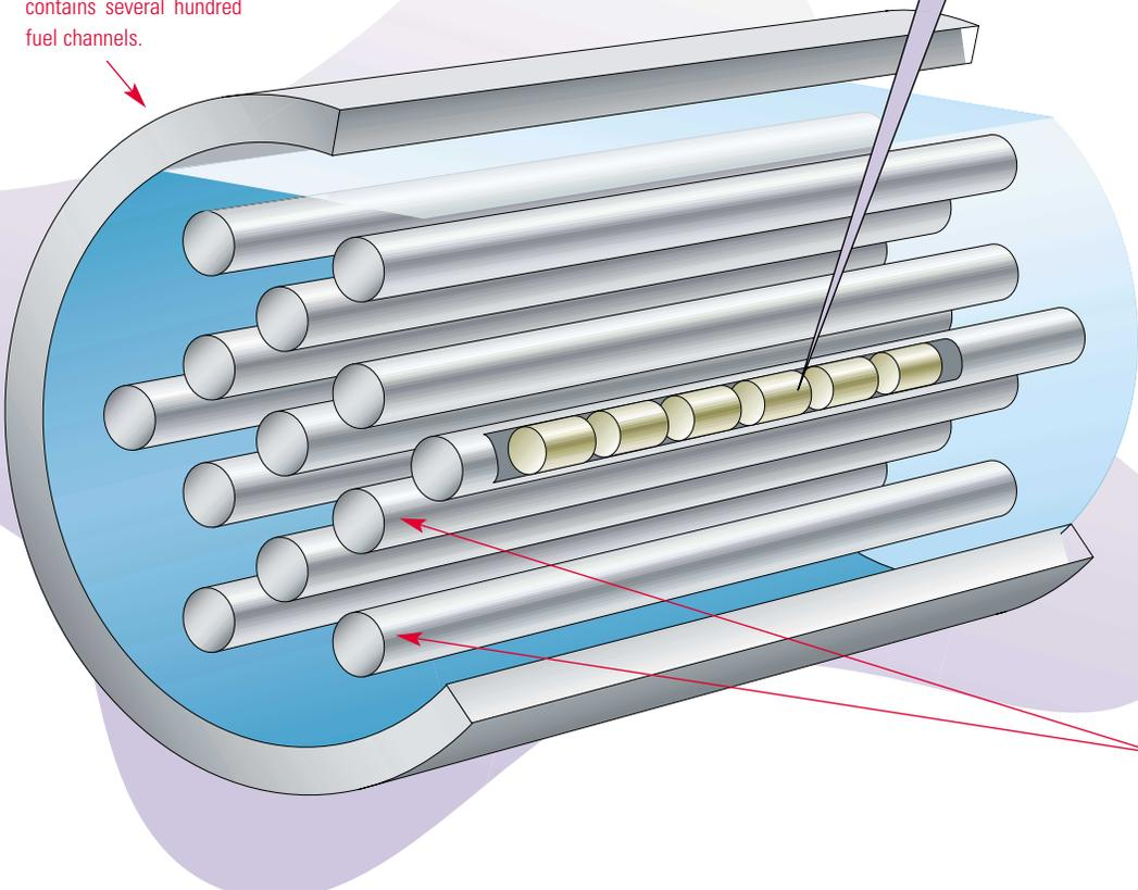
A **nuclear fuel bundle** is made up of several metal tubes, each housing uranium fuel in the form of **ceramic pellets**.
